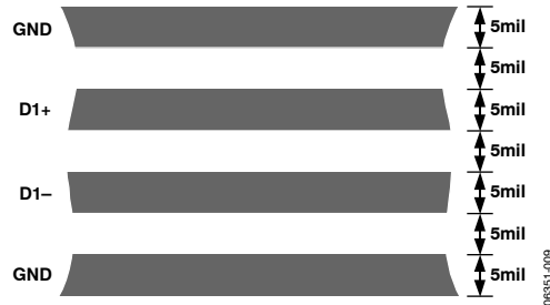
Figure 18. Arrangements of Signal Tracks
